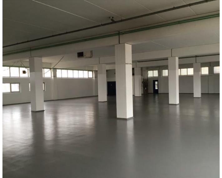
*Stonclad GS, a troweled epoxy mortar system, provides this production facility with superior impact, abrasion and chemical resistance. Stonglaze VSR and VSD protect the walls from splashes, spills, fumes and abrasion.*
