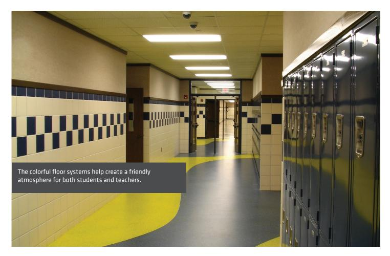
shapes in an endless palette of colors. The use of a unique urethane aggregate in place of the customary marble used in terrazzo produces much quieter floors and eliminates echoes and reverberation.
